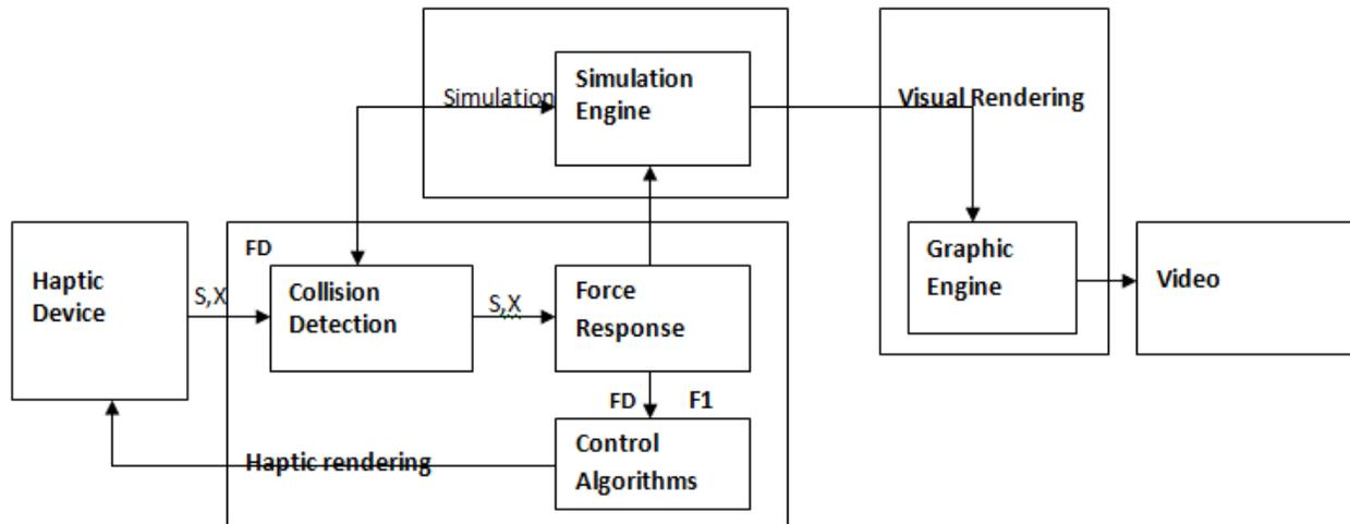
Figure 3: Haptic system block diagram
