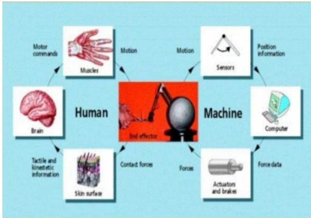
Figure 1: Basic Configuration of haptics
